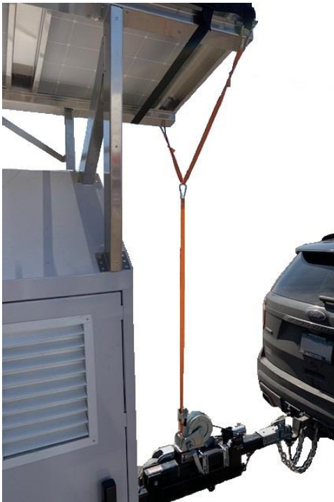
Front Solar Tie-Down Configuration
