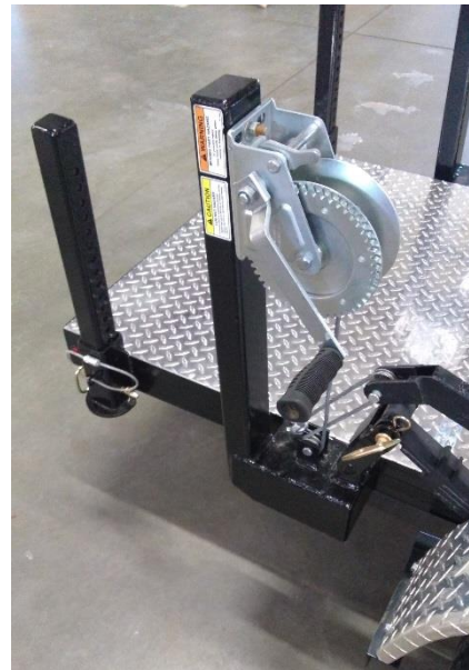
Rear Winch and Leveling Leg
