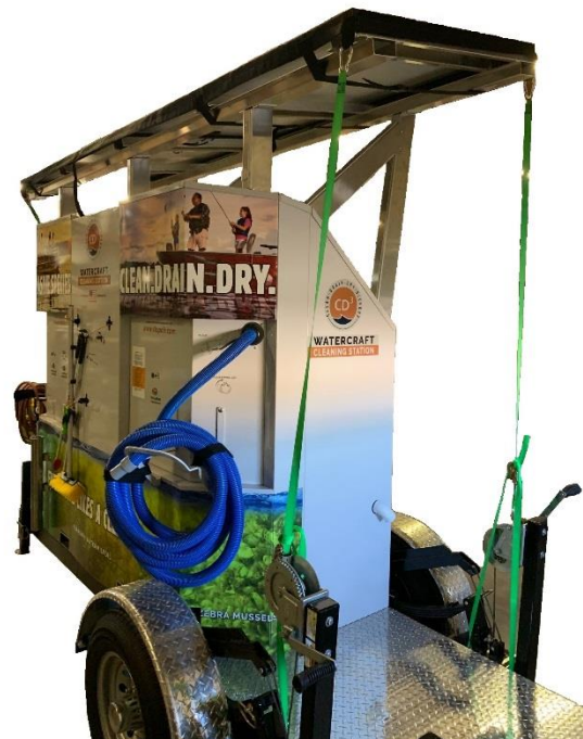
Rear Solar Tie-Down Configuration
